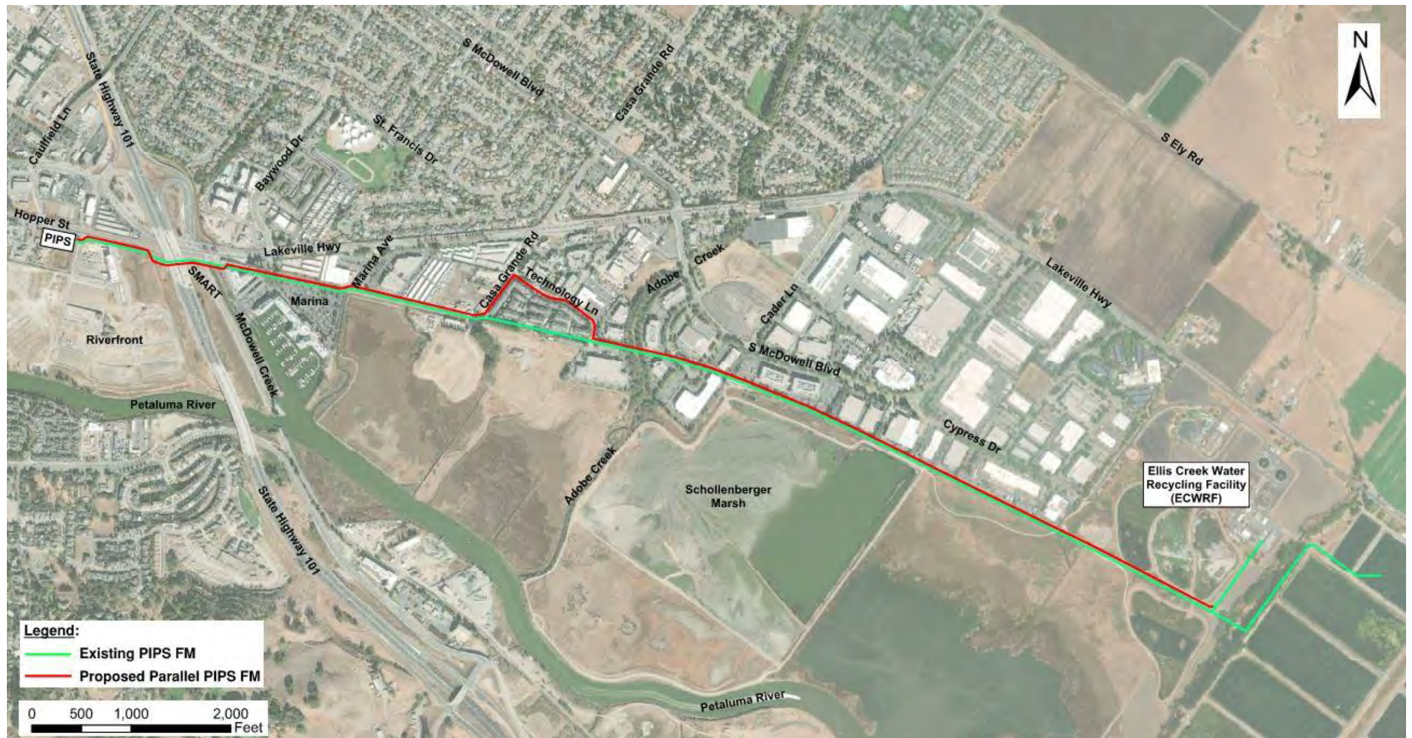
Figure 2-1: Existing Force Main and Proposed Parallel Force Main Alignment Overview
