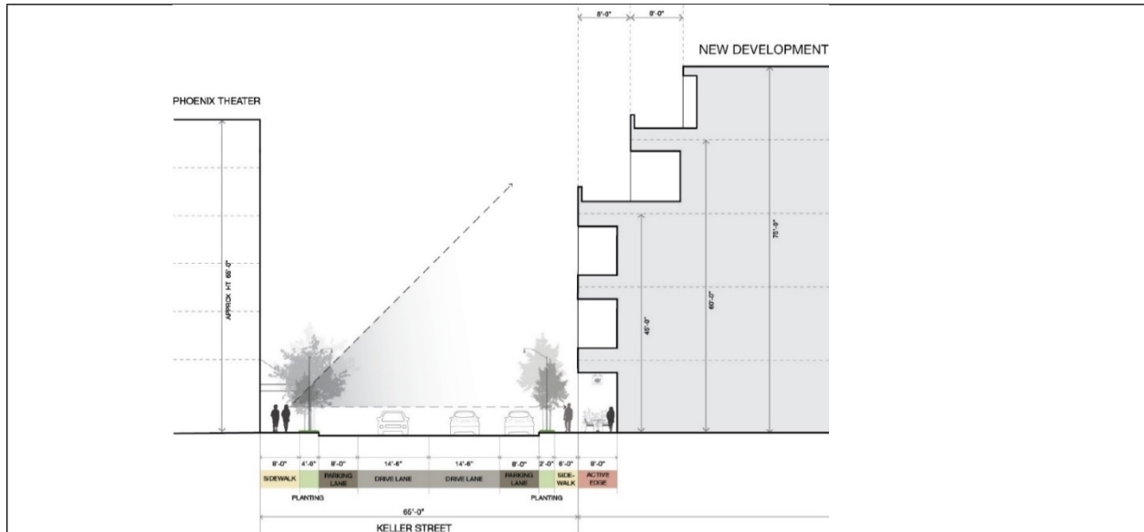
Figure 10.1: Line-of-sight analysis to depict the pedestrian-level view on Keller Street to show the stepbacks that apply to the front of a building above 45 feet.
