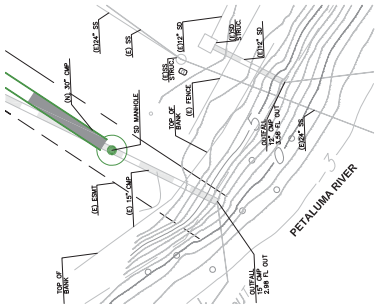
HAYSTACK STORM DRAIN OUTFALL DETAIL
