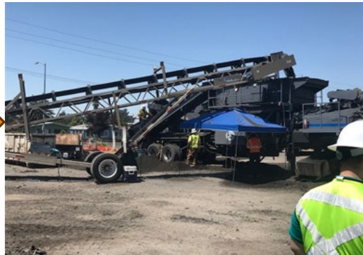
Step 2 Processing with asphalt emulsion (Cold Central Recycling Plant)
