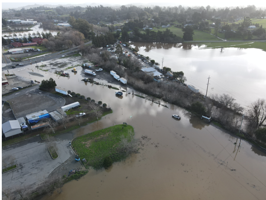
Image 3: The third in another aerial taken on January 10, 2023 showing what happens to flood flows directly downstream of the intersection of Rainsville Road and Stony Point Road. The River is out of bank and flooding outward from both banks. On the right the flooded pasture fronts on Bailey Avenue and the entire right-of-way of Stony Point Road is underwater, widening out onto the adjacent private property. Gravel placed as fill and compacted into parking lots has been placed on both sides of the River constricting its flow. The result is the widening and deepening of the water flowing from upstream created at the confluence of WillowBrook Creek coming under Stony Point and Highway 101 from the northeast with the Liberty/Marin/Wilson Creeks that flow around and across the KOA property. (Source: Pam Tuft, 2023)
